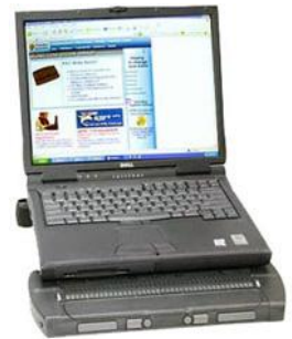
A convector that translates regular text into Braille.
